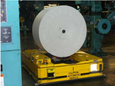
The photos above show the old AGV system carrying a roll and waste bin.
